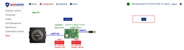
Click the **Test** button to test the signs. The highlighted signs will flash for approximately 30 seconds.
