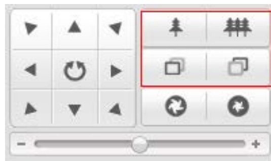
Figure 2-11 Zoom / Focus Adjustment Via PTZ Interface
