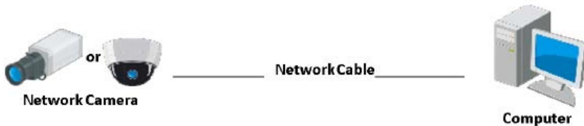
Figure 3-1 Connecting Directly
